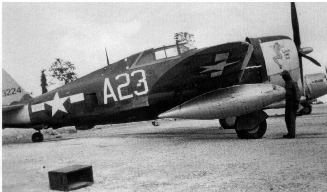
"SLEEPY TIME GAL" was a P-47D-15-RA assigned to the 69th FS, 58th FG and flown by 1Lt Herbert B. Emrich. The white cowl and letter 'A' on the fuselage side were used as squadron markings by the 69th FS. A portion of the canopy frame appears to be painted yellow. The Jug is carrying natural metal P-38 style drop tanks.
