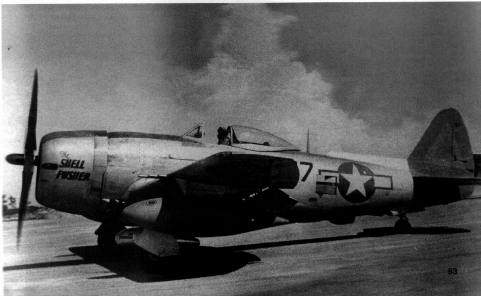
(Below) The SHELL PUSHER was a P-47N-1-RE (#107) flown by Capt Robert Forrest of the 463rd FS, 507th FG while stationed on Ie Shima during the summer of 1945. The Jug is taxiing forward bearing the weight of two 165 gallon wing drop tanks and a centerline 75 gallon drop tank. (Santiago A. Flores)
