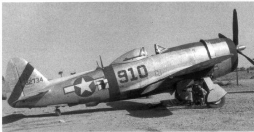
(Above) Ground crews attend to the turbosupercharger intake ducting on this P-47D-30-RA assigned to the 91st FS, 81st FG. The 81st FG was assigned to the 14th AF in China where it operated in the ground attack role against Japanese forces in northern Burma and southern China in 1944 and 1945. (George McKay)
