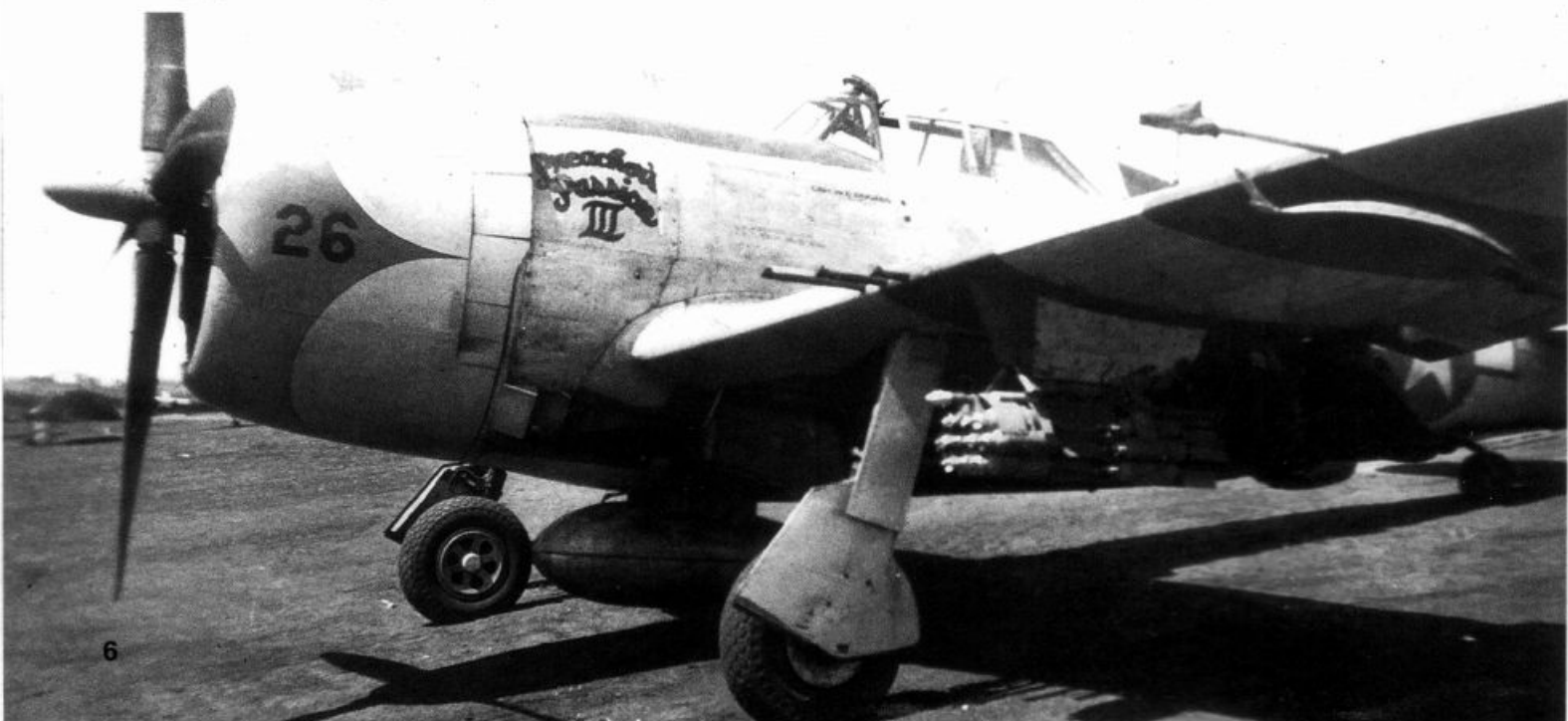
(Below) Lt Bill Rogers of the 39th FS, 35th FG flew Preacher's Passion III. The P-47D is carrying a fragmentation cluster bomb on the wing pylons and a 75 gallon drop tank on the centerline station.
