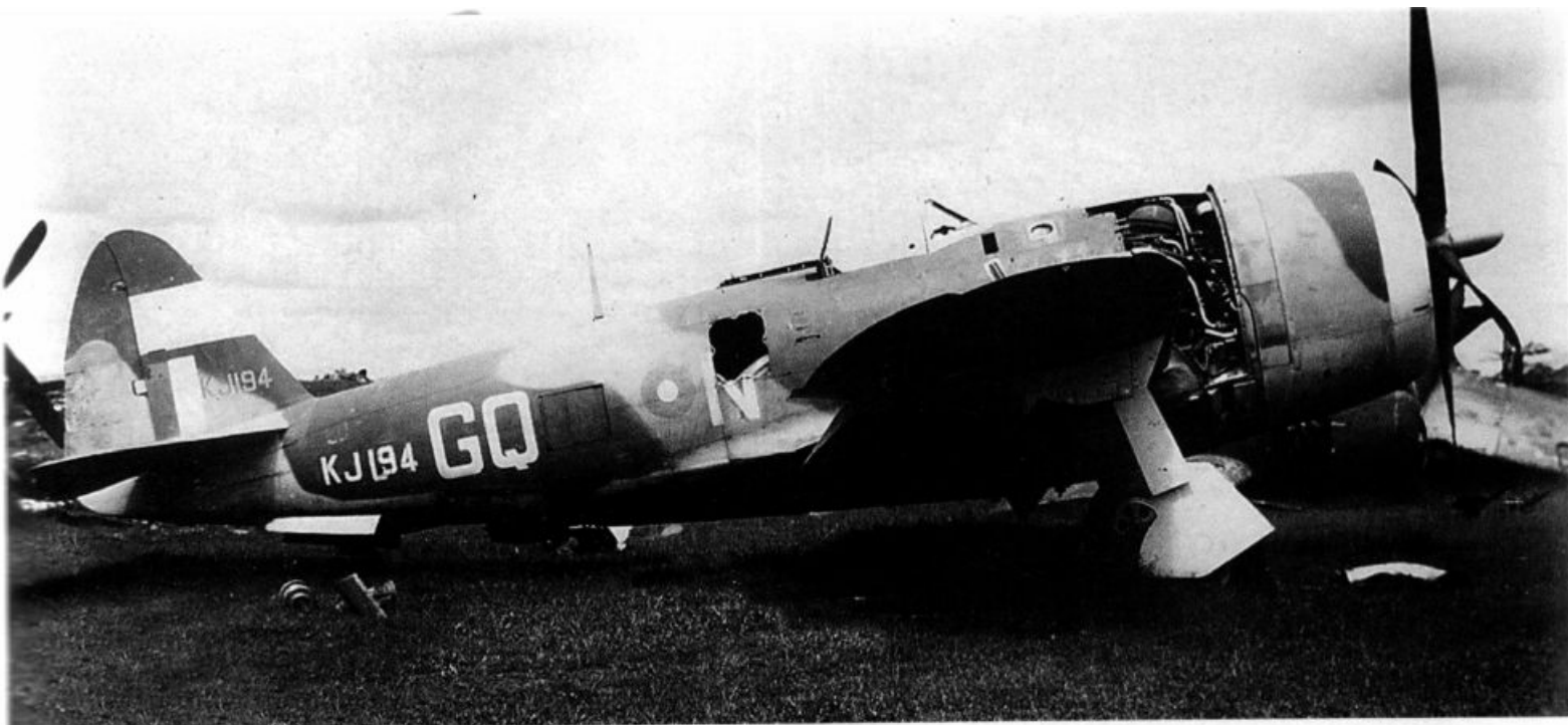
(Above) A somewhat dilapidated Thunderbolt Mk II undergoes maintenance in Burma in 1945. The Jug was assigned to No. 134 Squadron and was camouflaged with Dark Green and Dark Earth upper surfaces and Medium Sea Grey undersides. White wing, tail, and cowl ring ID bands were carried by all camouflaged SEAC Thunderbolts. (R.C. Jones)
