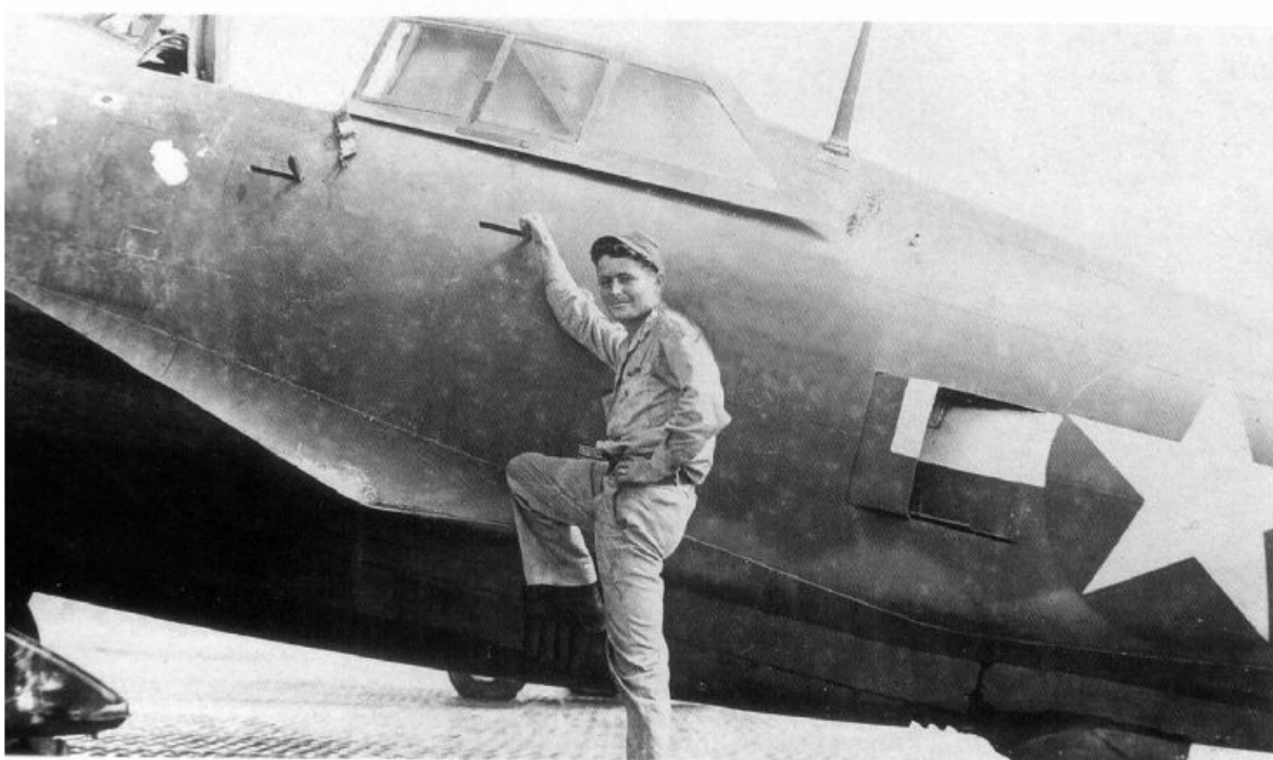
(Above) Lt William B. Foulis of the 341st FS, 348th FG scored six kills while flying the Jug. One victory was a twin engine Mitsubishi Ki-46 Dinah reconnaissance aircraft while the remaining five were single engine fighters. The P-47 was equipped with a pull down step and a pair of fold out hand-holds to help the pilot get aboard. Mountain climbing skills were no doubt helpful when laden with a Mae West, parachute, and survival equipment.
