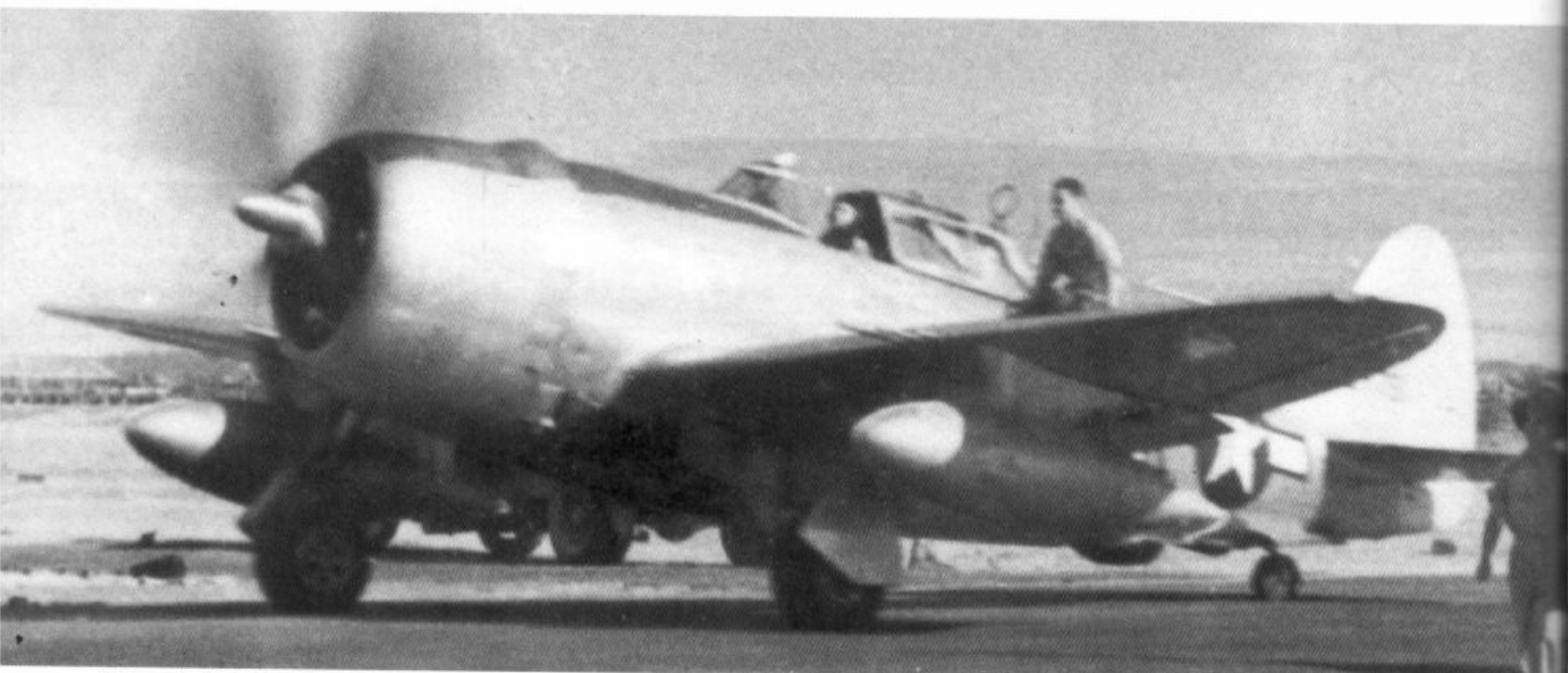
(Below) Carlotta was a weathered P-47D-21-RE assigned to the 88th FS, 80th FG at Barrackpore, India in March of 1945. An olive drab Jug at this stage of the war was rare — most 80th FG P-47s were natural metal. (P.M. Bowers)
