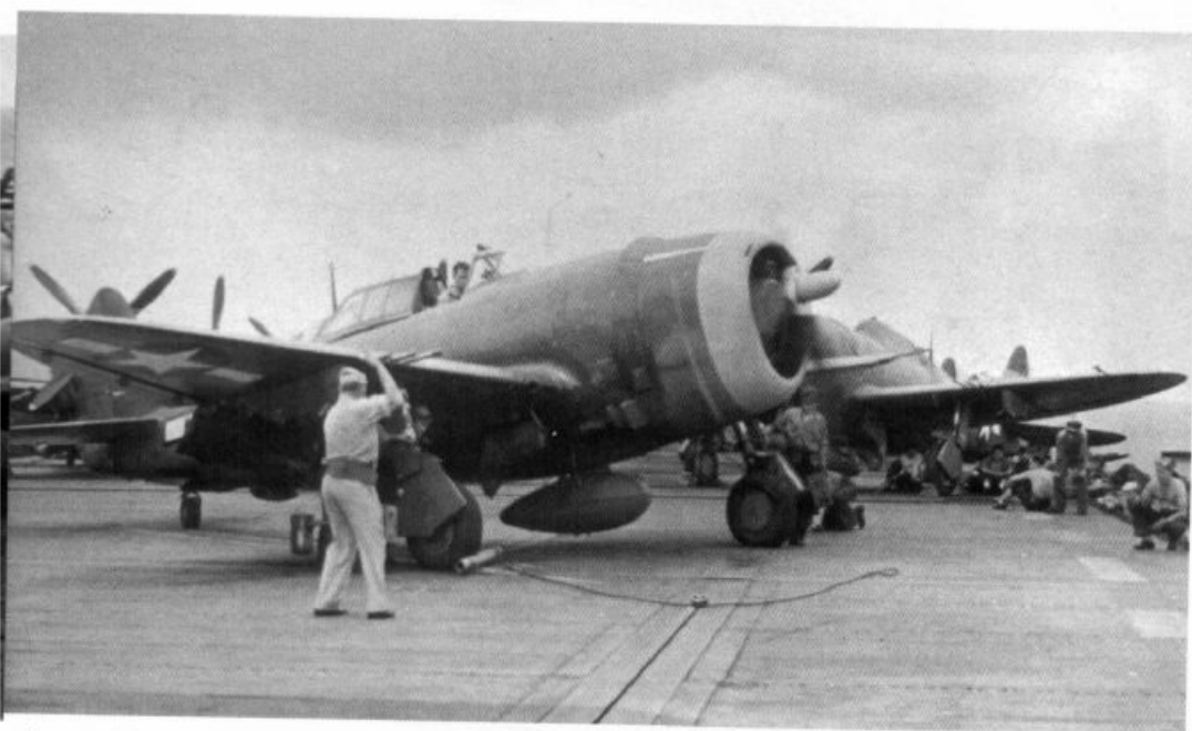
One by one, the P-47s are brought forward to the catapult. The catapult bridle rests on the deck in the foreground.
