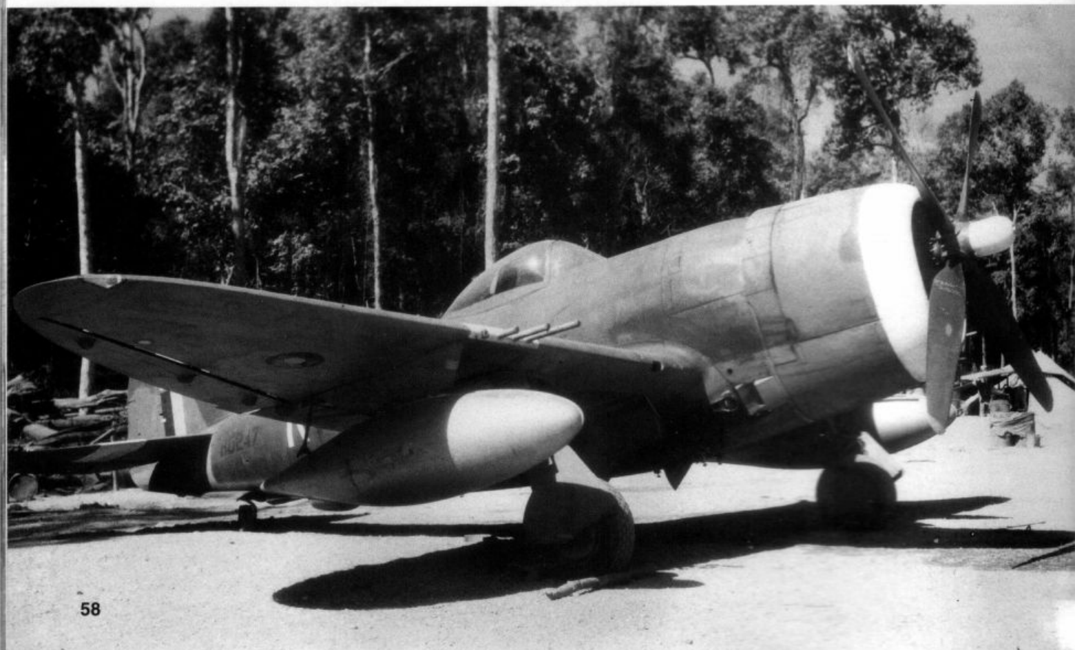
(Below) This Thunderbolt II (K*N*V/HD247) of No. 79 Squadron is equipped with a Hamilton-Standard Hydromatic propeller and carries 165 gallon drop tanks under the wings. The original RAF red, white, and blue roundels were changed to dark blue and light blue and reduced in size because they were too conspicuous — then SEAC HQ mandated the use of large white ID bands on the cowl, wings, and tail surfaces... (K.M. Sumney via P.M. Bowers)
