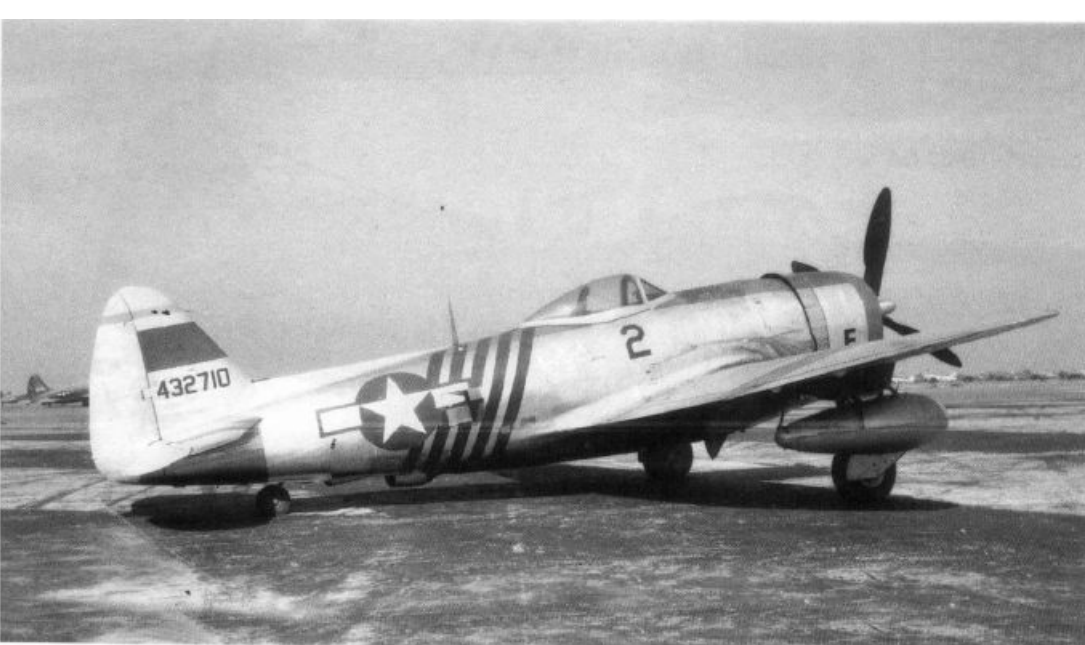
The 1st ACG received the new P-47D-30-RA before converting to North American P-51D Mustangs in early 1945. This natural metal Jug lacks the usual DF loop on the fuselage spine. (P.M. Bowers)
