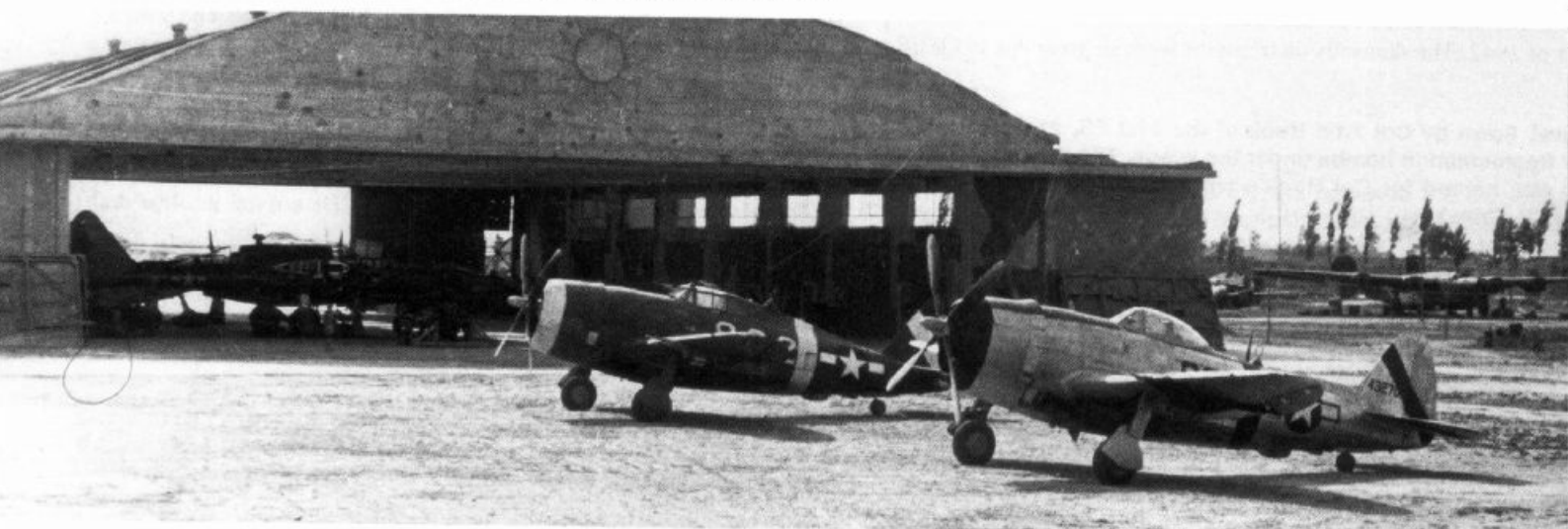
(Above) A pair of Thunderbolts assigned to the 91st FS, 81st FG, are parked in front of a hangar at a field in southern China. The natural metal Jug is a P-47D-30-RA. Both P-47s are equipped with DF loops on the fuselage spine and feature the standard ID bands for camouflaged and natural metal Jugs operating in the CBI. (L. Davis)
