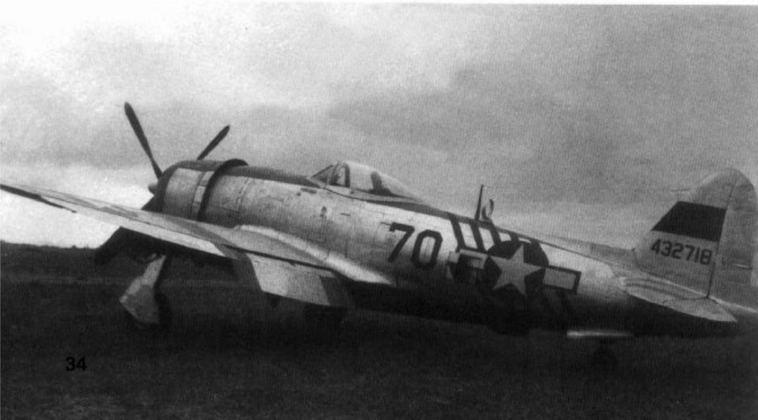
This P-47D-30-RA is equipped with a DF loop for operations over the inhospitable terrain of northern Burma and southern China. The five dark blue fuselage stripes of the 1st ACG were instantly recognizable to friend and foe alike.
