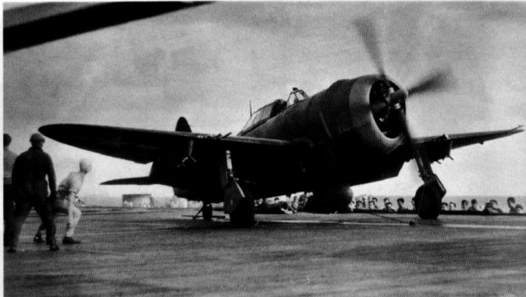
Once hooked up, the slack in the bridle is taken up, the engine brought up to full power, and the Thunderbolt is shot into the air. US Navy deck crews were no stranger to the roar of the 18-cylinder P&W R-2800 engine — it also powered the Grumman F6F Hellcat and Vought F4U Corsair.
