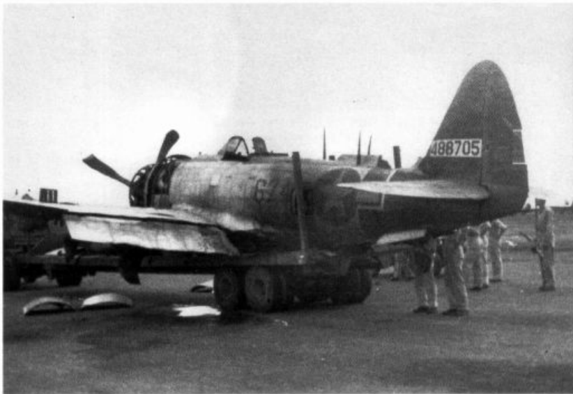
(Above) The pilot of this P-47N-1-RE (44-88705) jettisoned the canopy before landing wheels up on Iwo Jima. The Jug was hauled into the maintenance area for repair, but at this stage of the war the Thunderbolt may have been simply stripped for parts. (Larry Davis)
