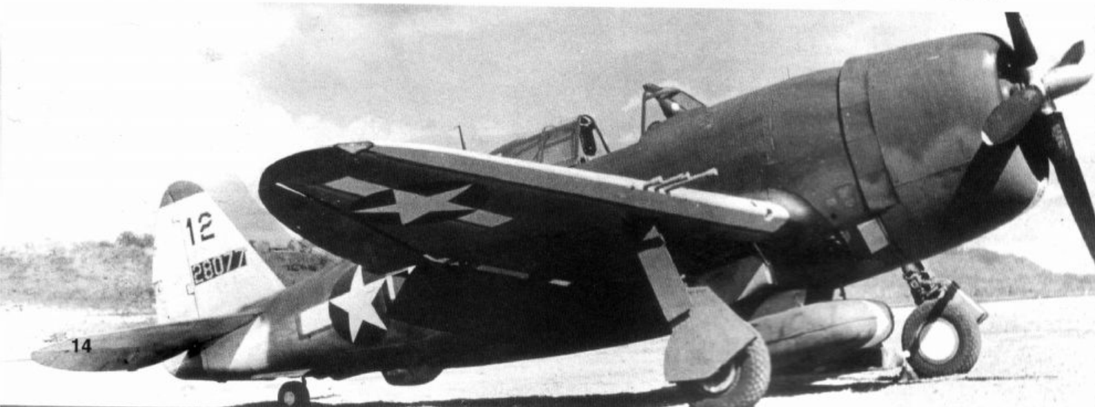
(Below) This P-47D-2-RE (42-8077) carries a 200 gallon drop tank on the centerline. The Jug has the white tail and wing leading edge stripes common to most Allied fighters in the SWPA. A white stripe has been added to the lower cowl and carried on to the drop tank. The aircraft number '12' has been repeated on the cowl stripe. This P-47 also appears to have a red surround to the fuselage insignia placing the time during the summer of 1943.
