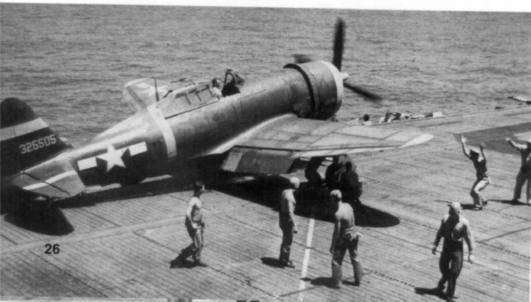
Once in position, the crews attach the catapult bridle to the Thunderbolt's landing gear struts and the holdback bar to the tail wheel.
