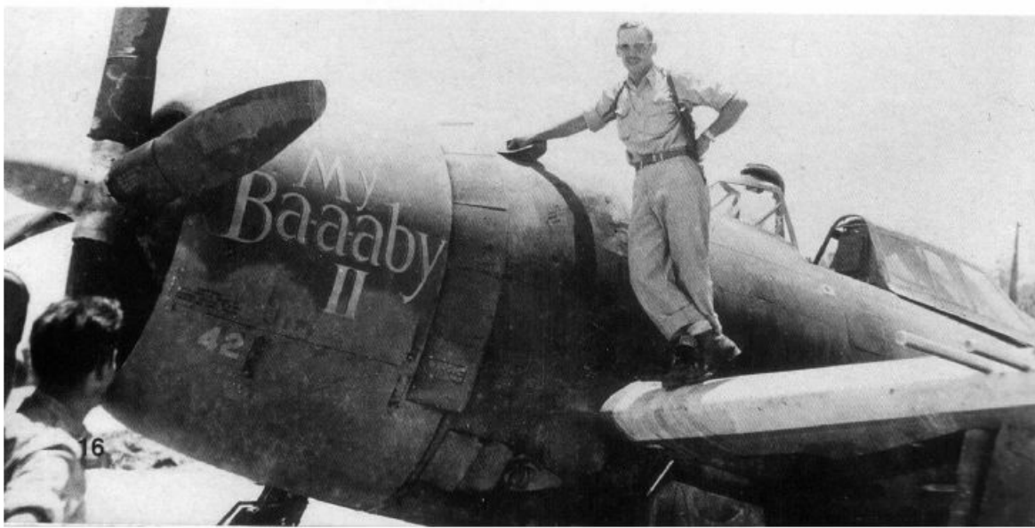
(Above) Lt William B. Foulis of the 341st FS, 348th FG scored six kills while flying the Jug. One victory was a twin engine Mitsubishi Ki-46 Dinah reconnaissance aircraft while the remaining five were single engine fighters. The P-47 was equipped with a pull down step and a pair of fold out hand-holds to help the pilot get aboard. Mountain climbing skills were no doubt helpful when laden with a Mae West, parachute, and survival equipment.
