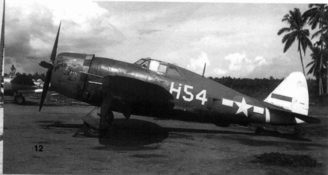
THE PIED PIPER was part of the 310th FS, 58th FG. The P-47D-16-RE (42-275885) has alternate yellow and olive drab cowl flaps and carries its nose art on a yellow cowl. (E.M. Sommerich via P.M. Bowers)
