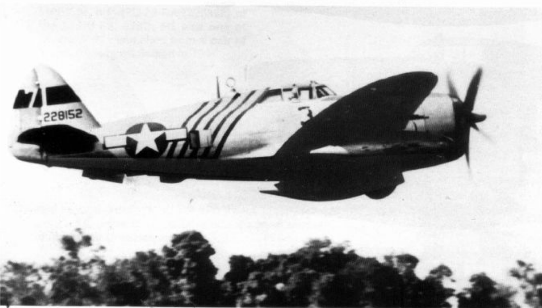
A P-47D-11-RE of the 5th FS, 1st ACG roars off the runway carrying a pair of P-38 style drop tanks. These tanks were popular among Thunderbolt units since they offered an increase in fuel over the standard 75 gallon tanks. The Jug wears a black '3' on the fuselage, but carries a white '71' on the black tail band.
