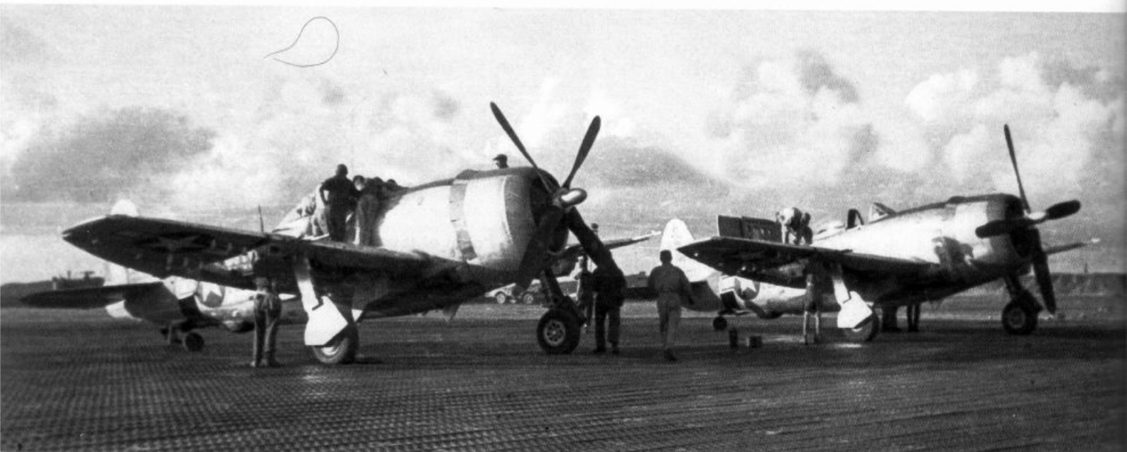
(Above) Mechanics and armorers of the 413th FS, 414th FG work on a pair of P-47Ns before a mission. Almost the entire outer wing panels of the P-47 was taken up by ammunition boxes used to feed the eight fifty caliber machine guns. Each box held up to 500 rounds. (George Lovering via Larry Davis)
