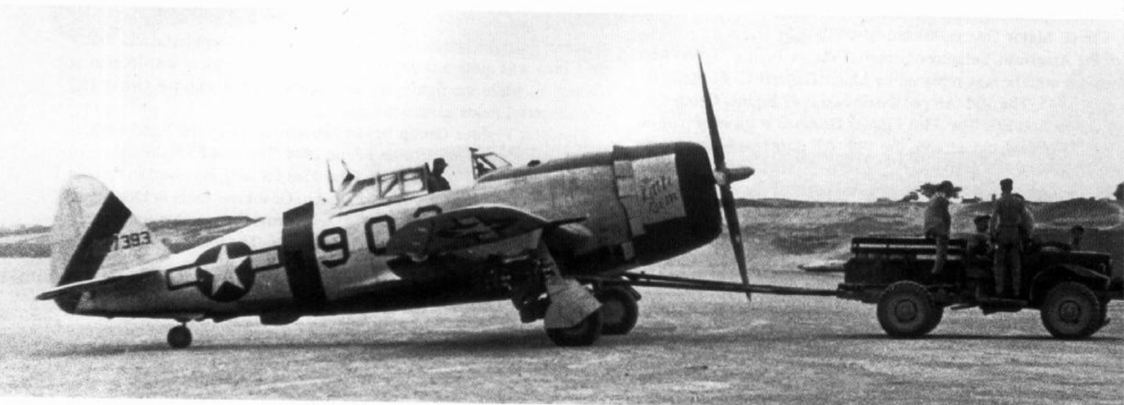
My Little Gem , a P-47D-23-RA (42-27393) of the 91st FS, 81st FG, is towed across the flightline while loaded with fragmentation bombs. It is not known if the My Little Gem refers to the Thunderbolt or the
