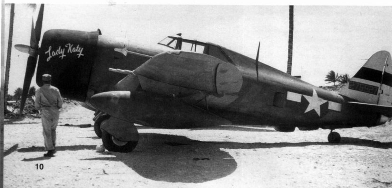
Lady Katy was a P-47D-16-RE (42-75927) assigned to the 9th FS of the 49th Fighter Group. This Thunderbolt wears a black painted cowl rather than the more usual white. A black band is also applied across the tail. The Jug is carrying the popular 165 gallon P-38 style drop tanks on the wing pylons. (J.P. Gallagher)
