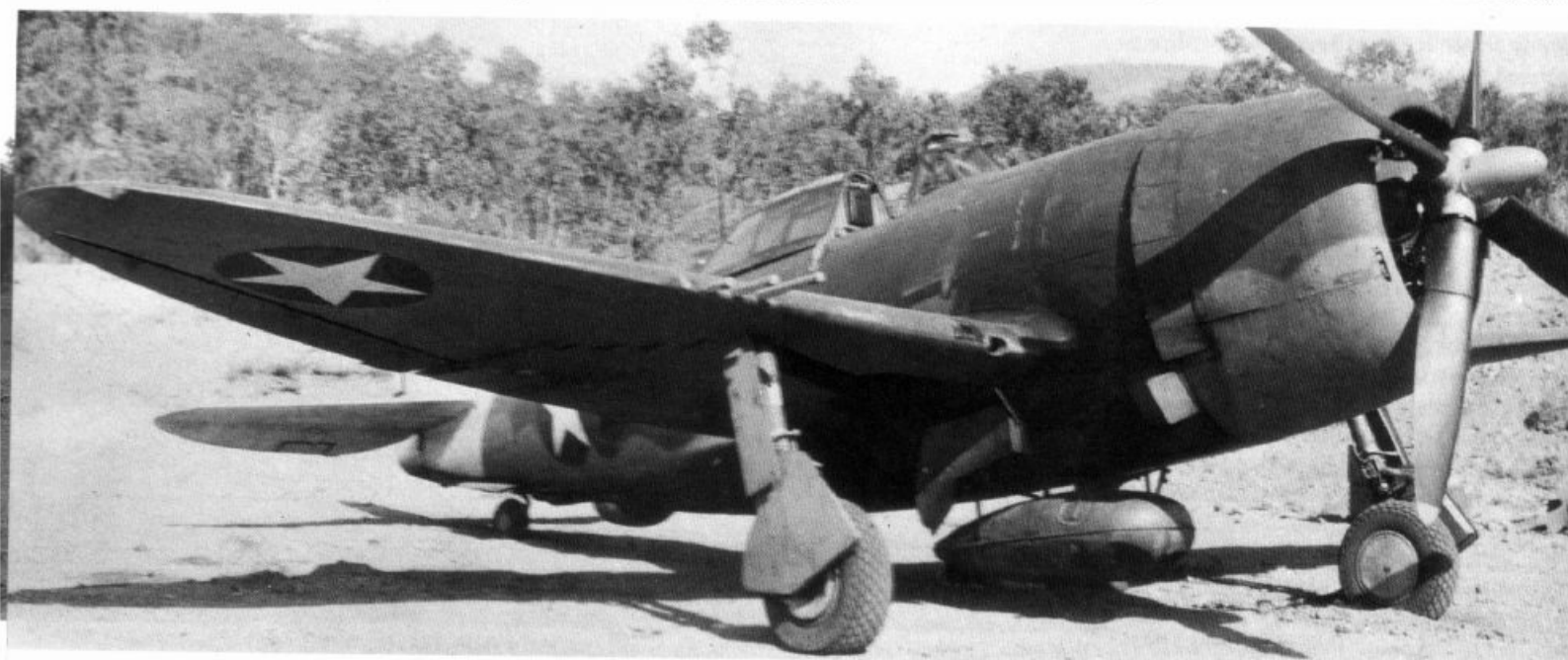
(Above) Early P-47Ds used by the 348th FG lacked wing pylons for bombs or drop tanks. This Jug does carry the flattened 200 gallon drop tank on the centerline and early style US insignia on the wings and fuselage. Early Thunderbolts also had straight cowl flaps which lacked the scallop on the lower two flaps.
