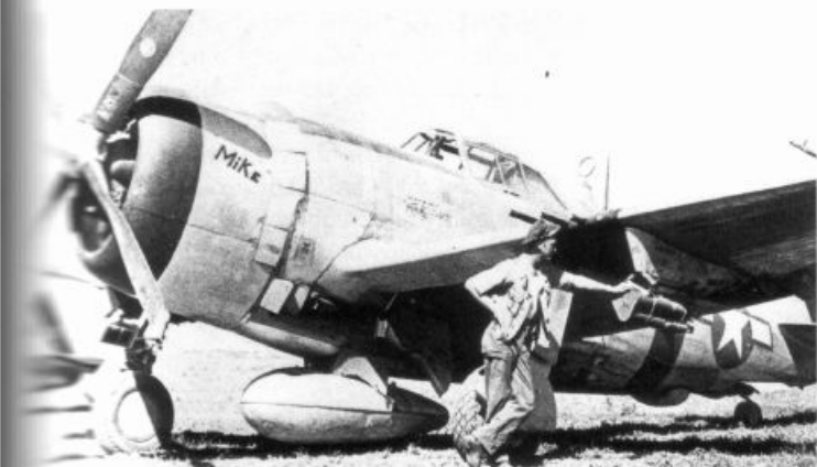
"Mike" was a P-47D-5-RA assigned to the 464th FS, 507th FG while the Group was in China as part of the 7th AF. The Jug is armed with fragmentation cluster bombs on the wing pylons and a 110 gallon fuel tank. For some reason, "Mike" is shod with tires having two different tread styles. (Larry Davis)
