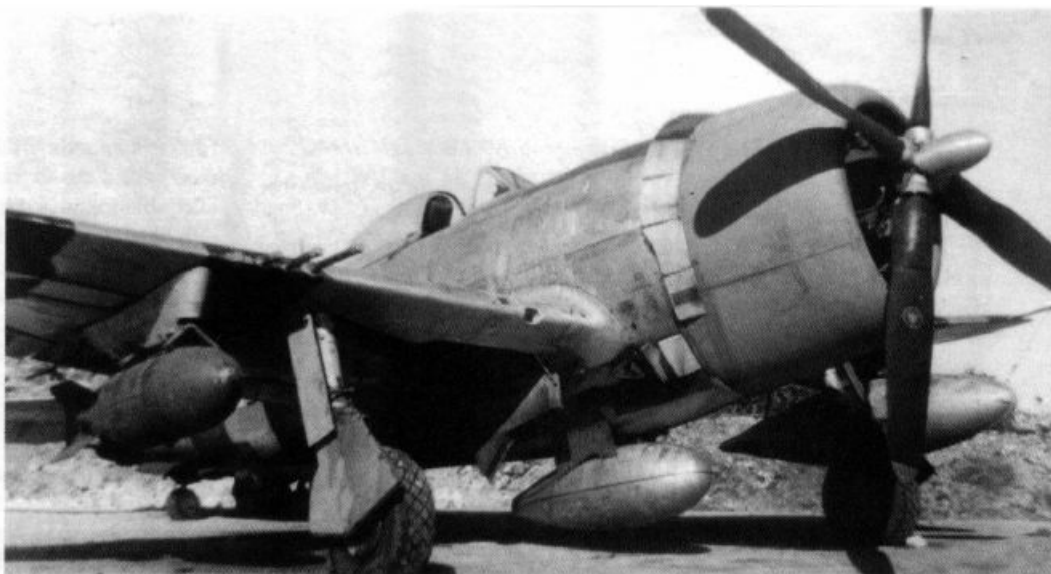
Lt Robert Knight flew this P-47D-25-RE while assigned to the 310th FS, 58th FG in Okinawa. The Jug carries an asymmetrical load of one 1000 lb bomb under the starboard wing pylon and one 165 gallon drop tank under the port wing. A 75 gallon tank is mounted on the centerline rack. Knight finished the war with two victories. (Peter Kampman)
