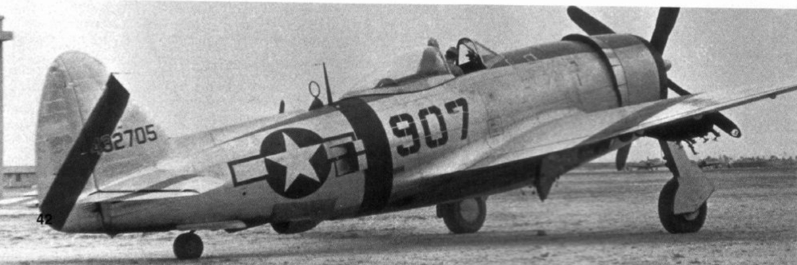
(Above) A pair of Thunderbolts assigned to the 91st FS, 81st FG, are parked in front of a hangar at a field in southern China. The natural metal Jug is a P-47D-30-RA. Both P-47s are equipped with DF loops on the fuselage spine and feature the standard ID bands for camouflaged and natural metal Jugs operating in the CBI. (L. Davis)
