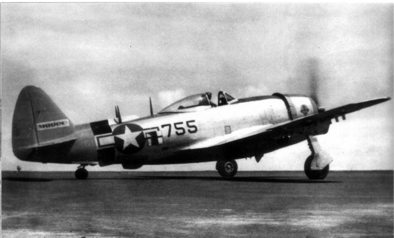
(Above) A P-47N-1-RE Thunderbolt of the 456th FS, 414th FG slowly taxis forward after returning from a mission in late July of 1945. The dorsal fin fillet on the aft fuselage provided additional side area to help counter the increased power and torque from the engine. (Larry Davis)
